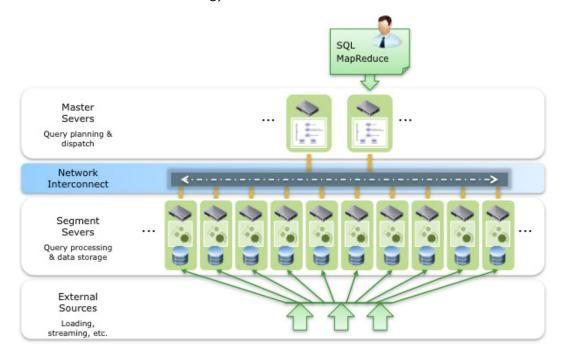
Figure 2. Greenplum Database MPP architecture
